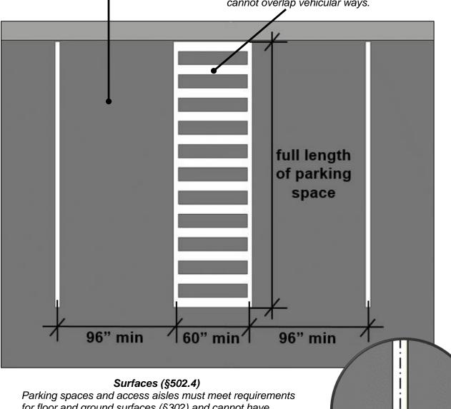
for floor and ground surfaces (§302) and cannot have changes in level other than slopes not exceeding 1:48.
