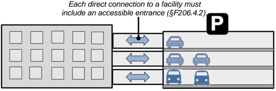
Dispersing accessible spaces among accessible entrances requires placement of non-van accessible spaces on different levels. All van spaces can be grouped on one level (§F208.3, Ex. 1).
