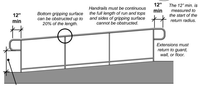
Extensions with a leading edge 27" high max. can extend any amount from posts. Those with a leading edge higher than 27" are limited to a 12" protrusion from posts (§307.3). The sloping portion of handrails are not required to comply with requirements for protruding objects.
