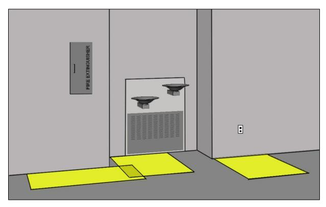
Clear floor space is required at each accessible element, including storage cabinets, drinking fountains and other fixtures, and electrical outlets. Clear floor spaces can overlap where elements are in close proximity.
