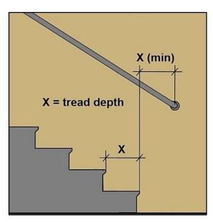
Handrails at the bottom must extend beyond the last riser nosing at the slope of the stair flight for a distance at least equal to one tread depth or be continuous to the handrail of an adjacent stair flight protruding objects.
