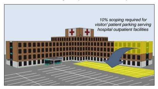
Within a multi-use facility, the 10% requirement applies to the number of visitor/ patient spaces intended to serve hospital outpatient facilities. Most local zoning codes require parking spaces based on facility square footage, occupant load, and occupancy and can be consulted when determining the number of spaces serving outpatient facilities. Spaces serving employees or other areas of a hospital are subject to the regular scoping table.
