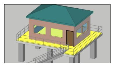
The 500 sq. ft. maximum applies to the gross floor area, including exterior floor space, of all press boxes serving a playing field, stadium, or other assembly area. If a site has multiple assembly areas with press boxes, the aggregate area of press boxes is to be calculated separately for each assembly area.
