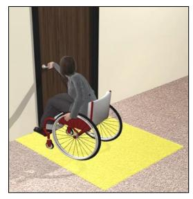
Required door clearances provide unobstructed space for maneuvering through doorways.
