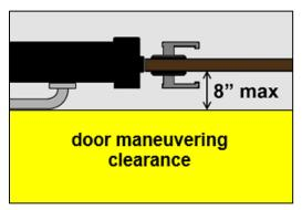
Handrails and other elements cannot overlap the door maneuvering clearance but can be located within the 8" max. offset from the face of the door.
