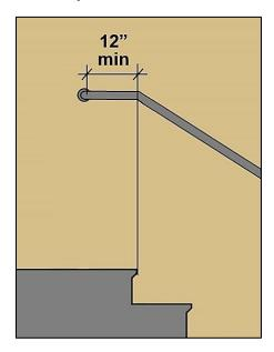
Handrails at the top of stairways must extend 12" minimum horizontally above the landing beginning directly above the first riser nosing or be continuous to the handrail of an adjacent stair flight (§505.10.2).
