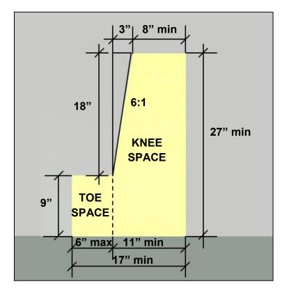
Where knee and toe space is required at an element, it must be at least 17" deep.
