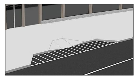
At least 1 accessible passenger loading zone is required in every continuous 100 linear feet (or fraction) of passenger loading zone space.
