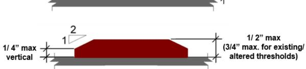
Note: vertical edge must be located below bevel, not above
