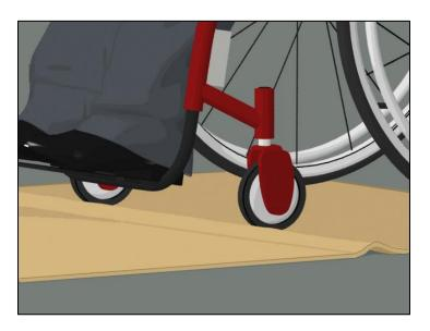
Exposed edges must have trim on the entire length of the exposed edge and be fastened to the floor to prevent curling. Trim must meet specifications for changes in level, including requirements for beveled edges when the height exceeds ¼ inch. The maximum height is ½ inch.
