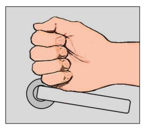
Operability with a closed fist is a reliable test of usability, but is not required by the standards.
