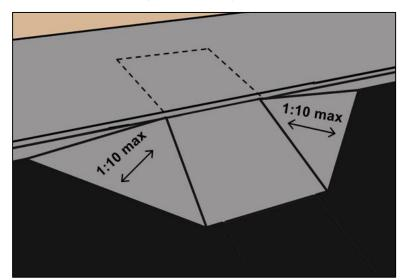
Side flares can be provided to prevent tripping hazards. Edge protection is not specified for curb ramps.
