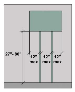
Objects with leading edges 27" maximum or above 80" can protrude any amount from posts or pylons.
