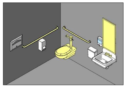
In a restroom project involving alterations to the toilet, grab bars, faucet controls, and mirror, the standards apply to these elements but not to those that remain unaltered. In more extensive projects where additional elements are altered, application of the standards is greater, commensurate with the scope of work.
