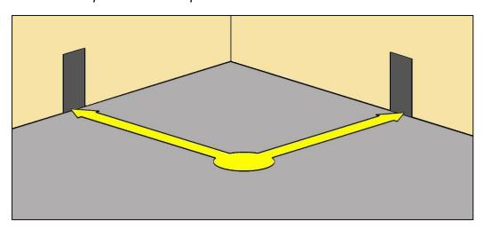
Accessible means of egress can share a common path of egress travel as allowed for means of egress by the applicable building or life safety code (§F207.1).
