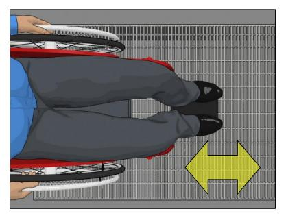
Elongated openings, like those of most grates, must be oriented so that the long dimension is perpendicular to the dominant travel direction. In locations where there is no dominant flow pattern, openings must be limited to ½" in both dimensions. Where an accessible route is available to bypass openings completely, they can be oriented in any direction.
