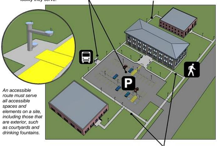
An accessible route from public streets and sidewalks must connect directly or indirectly to all accessible facilities and elements on a site.
