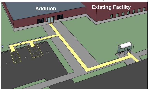
At least 1 accessible route is required from site arrival points (accessible parking, passenger loading zones, public streets and sidewalks, and transit stops, where provided) to an accessible addition entrance. If the addition does not have its own entrance, an entrance of the existing facility must be made accessible to serve the addition and an accessible route must serve all accessible spaces and elements of the addition.
