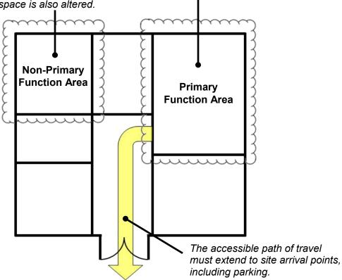
If alterations are limited only to elements in a room or space, then the standards apply only to the elements altered. Similarly, where spaces are altered, the standards apply to those spaces that are altered. If a room or space is completely altered (or built new as part of an alteration), the entire room or space is fully subject to the standards. Compliance is required to the extent that it is technically feasible.
