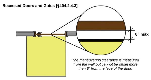
Thick walls, casework, shelving, columns and other elements can cause doors or gates to be recessed. If any obstruction within 18" of the latch side projects more than 8" from the face of a door or gate, maneuvering clearances for a forward approach must be provided. This space must be inset at obstructions so that it is no more than 8" from the face of the door or gate.
