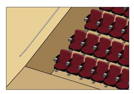
Handrails on assembly area ramps can be discontinuous and lack extensions to allow access to seating and to permit crossovers within aisles. (§505.3, §505.10)
