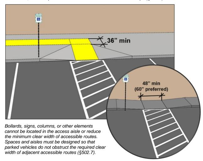
Where space for curb ramps is limited, including in alterations, parallel ramps can provide an alternative.
