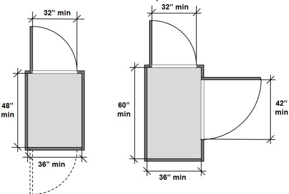
The clear floor space of platforms must be 36" wide min. If doors/gates are on the narrow end only, the length is 48" min. If a door/gate is on the longer side, the min. length is 60" to accommodate side approach maneuvering.
