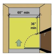
On the pull side of hinge approaches, 36" min. latch-side clearance is required if the depth is 60" min. (The depth can be 54" min. if the latch-side clearance is at least 42".)
