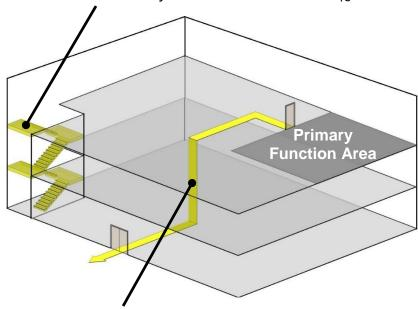
As necessary to achieve an accessible path of travel to a primary function area that is altered unless the cost is more than 20% of the cost of the overall alteration (§F202.4).
