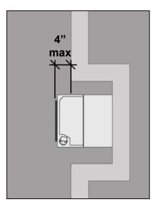
Elements, such as wheelchair accessible drinking fountains, must provide a knee clearance of at least 27". If located to provide, but not exceed this clearance (27" above the floor or ground absolute), they are not protruding objects because the leading edge will be within cane detection.
