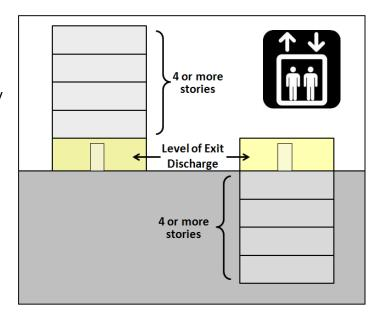
Only one of two accessible means of egress can contain an elevator with standby power
