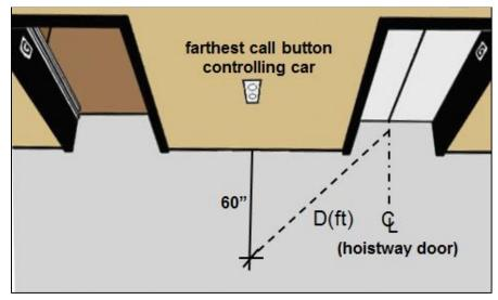
Minimum timing from car arrival notification to start of door closing: D / 1.5 ft/s (no less than 5 sec.)
