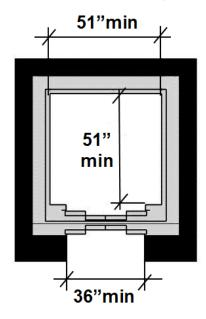
Alternative dimension permitted if the door has a clear width of 36" min.
