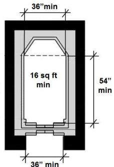
(32" min if door power operated and door/hoistway depth is 24" max )
