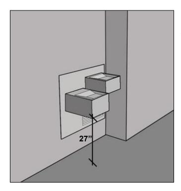
A wheelchair accessible unit located 27" absolute above the ground or floor is cane detectable and can be used to enclose one side of high units for standing access. In this instance, the 27" height is effectively an absolute dimension because it is the minimum required for knee clearance and the maximum specified for cane detection.
