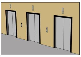
When an alteration is made to an existing car, it also must be made to all other cars that respond to the same hall call.
