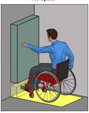
Objects that provide clearance for toes can overlap a portion of the clear floor space.
