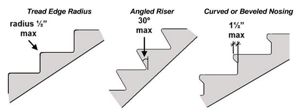
The radius of curvature at the leading edge of the tread must be ½" max.
