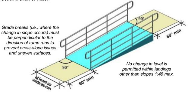
Intermediate landings between runs must be at least 60" wide clear and 60" long clear where ramps change direction (any change from linear). Handrails, edge protection, vertical posts and other elements cannot obstruct or overlap the minimum 60" by 60" clearance. The 12" minimum handrail extensions required at the top and bottom of ramp runs must be in the same direction of the run, but they can turn or wrap where handrails are continuous at the inside turn of dogleg or switchback ramps.
