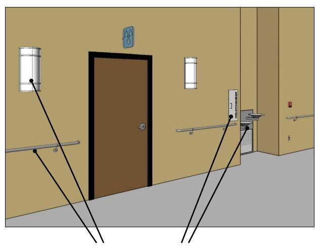
Sconces, handrails, cabinets, drinking fountains and other elements that project into circulation paths must comply with provisions for protruding objects (unless they are located within cane sweep or above headroom clearance). Requirements for protruding objects apply to all interior and exterior circulation paths of sites. They are not limited to hallways and corridors and apply equally to circulation paths in rooms and spaces.
