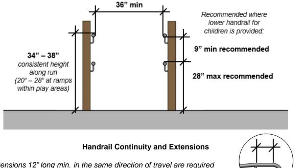
Extensions 12" long min. in the same direction of travel are required at the top and bottom of runs (except for inside rail of switchback ramps) to provide support before entering or exiting ramps.
