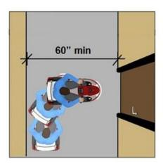
Space at least 60" deep in front of a door will accommodate a forward approach, except in case of hinge approaches on the pull side.
