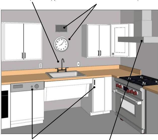
Appliance controls and handles to accessible storage are also covered as operable parts.
